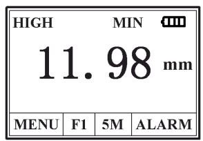
measurement carried out a moment ago, and the MIN indicator for the minimum value will flash several seconds. If you continue the measurement when the MIN is flashing, the former measurements will continue to take part in the min. value capturing. If you carry out measurement after MIN indicator stops flashing, the min. value capturing will begin from then on.
