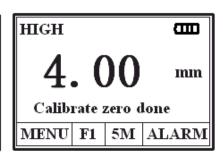
**Note:** After every change of the probe, probe temperature, ambient temperature changes, etc. After the work environment, or working for some time after the discovery measurement errors should see the standard test block measured value is accurate, if the difference would be larger school Zero operation.
