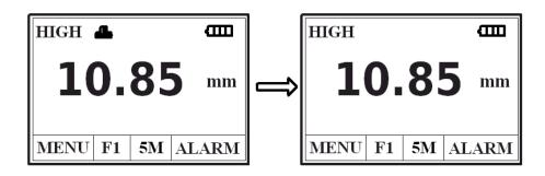
**Note**: when the probe is coupled with the material to be measured, the instrument will display the coupling indicator; if the indicator flashes or doesn't appear, it means that the coupling is not so good.
