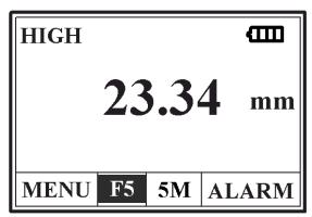
2) Press —, by pressing F1~F5 to display file No.s cyclically. You can exit by pressing or conducting one measurement.
