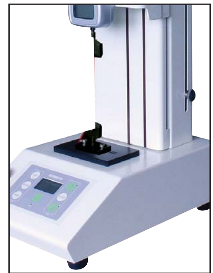
Stand with Optional Grip Performing Tension Test
