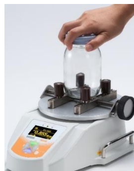
Opening/closing torque test of jar lid
