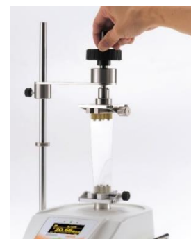
Twist test of screen protective film
