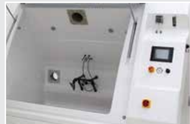
3 The Atmosfär chamber is now ready for other types of corrosion test.
