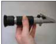
ACC100 Hand-held Salinity Refractometer
