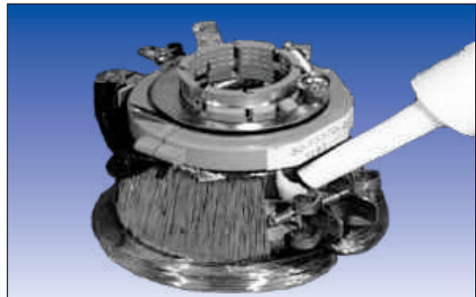
4460 Penetrates and Encapsulates a Tightly Wound Coil
