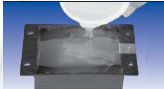
4461 Potting a Transformer for High Temp. Use
