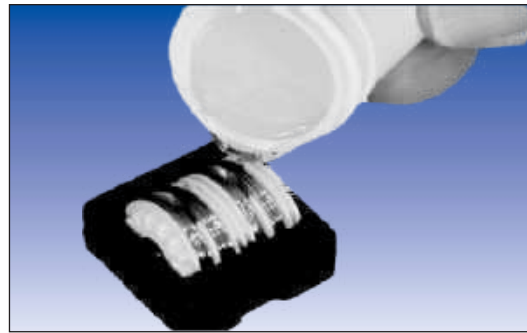
4460 Fully Impregnates a High Temperature Coil
